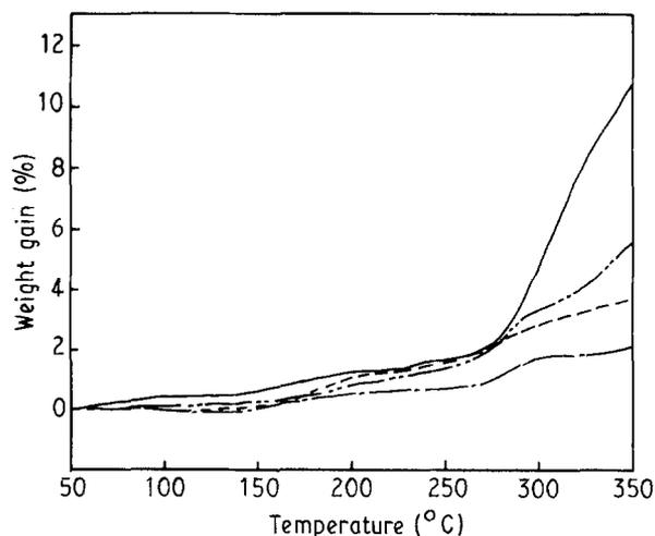
Figure 5 Effect of surface treatment on weight gain. Samples were treated with: ---, PAN; - · - ·, Si-epoxy; · · · ·, Ti-epoxy; —, untreated sample.
