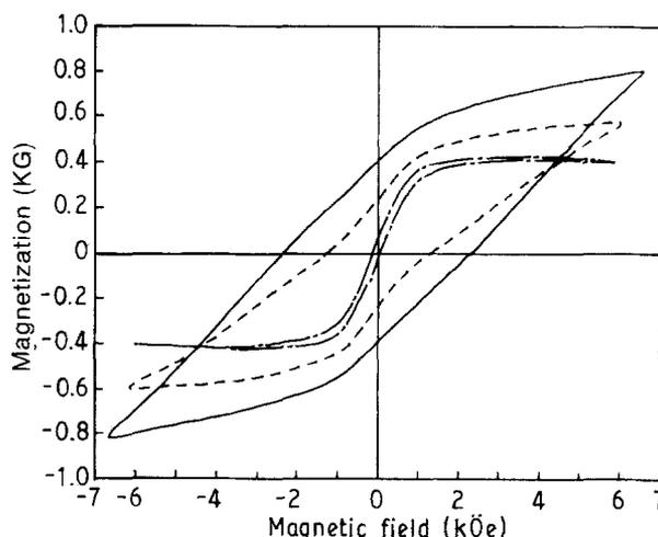
Figure 6 Demagnetization curves of plastic magnets oxidized in air for 10 h at  $200^\circ C$ . —, PAN-treated; ---, untreated; - · - ·, oxidized.
