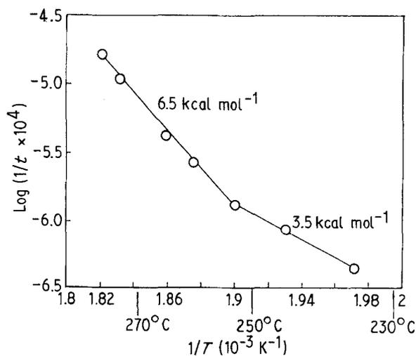
Figure 4 Arrhenius plot for untreated magnetic powders; reciprocal of time required for 1% weight gain versus reciprocal of absolute temperature.
